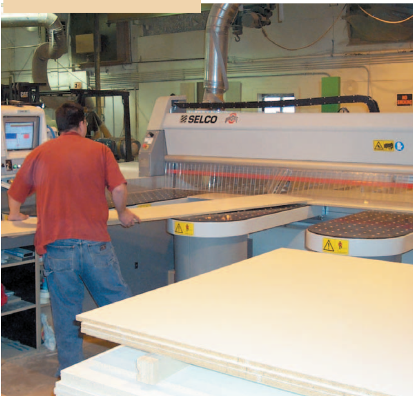
A Biesse Selco panel saw with labeling capability was recently added, and is the new key piece of equipment at the company.
